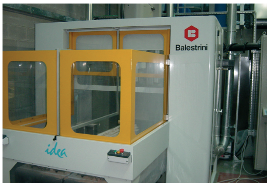
Photograph 1 CNC routing machine with interlocked doors
